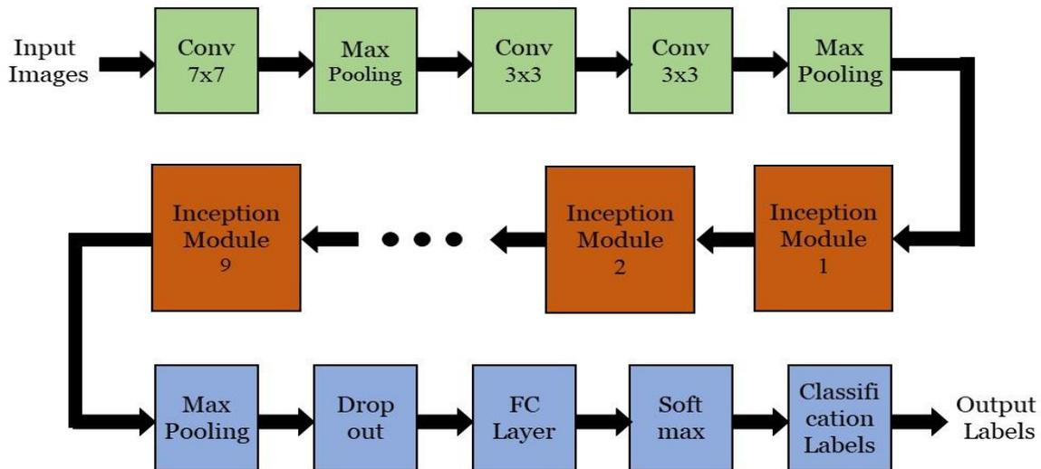
FIGURE 2. GoogLeNet architecture for NT region segmentation
