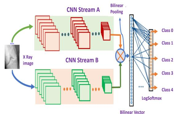
FIGURE 1. Architecture of Ortho Bilinear CNN Classifier
