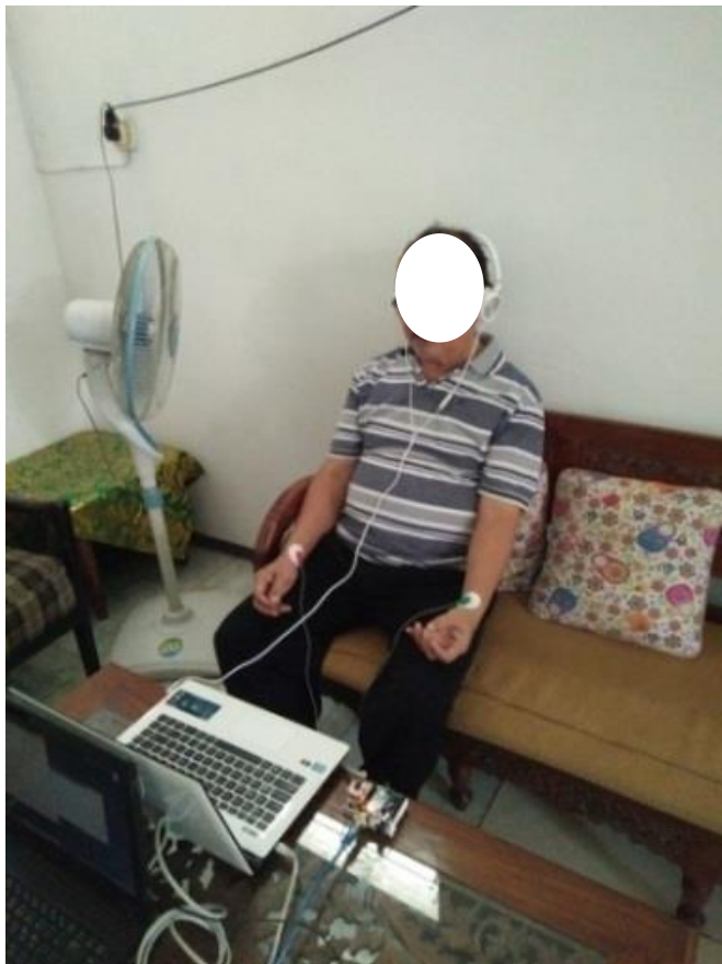
Fig. 4. Experimental setup showing ECG data acquisition using AD8232, Arduino Uno, and laptop interface.
